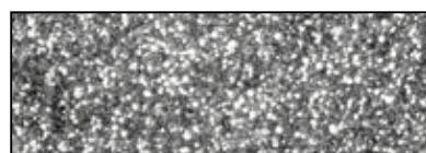
The fine uniform microstructure of ASP® carbide ensures superior strength
