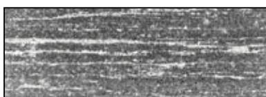
Conventionally produced HSS with a brittle carbide microstructure limits material strength
